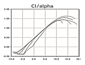
Fig.2 Coefficient of lift characteristics
