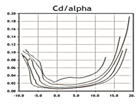
**Fig.3** Coefficient of drag characteristics
