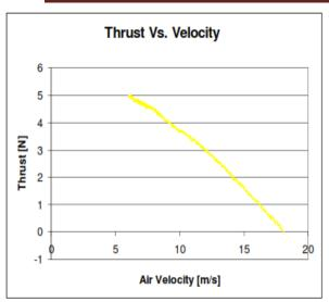
Fig.6 15"x10" Propeller. Thrust Vs. Velocity
